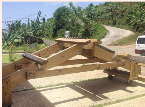
Mobile full-scale model of hurricane-resistant roof construction. Dominica 2017. Source: Dave Haption/IOM.
