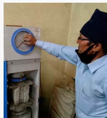
Block testing taking place at the Central Material Testing Laboratory in Nepal. Source: HRRP.
