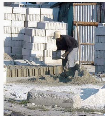
Low-strength blocks will affect compliance with standards. Source: UN-Habitat.
