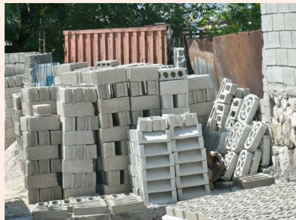
Low-quality blocks for reconstruction. Haiti. Source: UN-Habitat.
